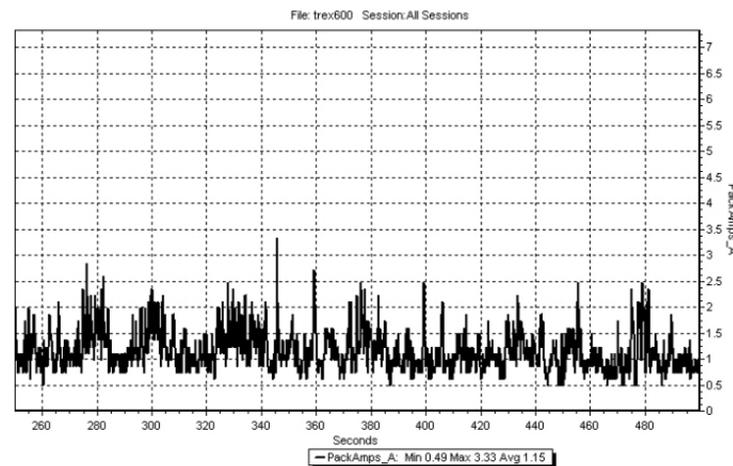
In the above example the average current was 1.15 amps, which calculates to 153mAh per 8 minutes (typical flight length). It's recommended that only 60% of the available capacity be used to ensure plenty of reserve battery capacity. In this example using 2000mAh batteries  $2000 \times 60\% = 1200\text{mAh}$  (available usable capacity) divided by the capacity used per 8 minute flight, 153mAh would allow up to 7 flights of 8 minutes each.
